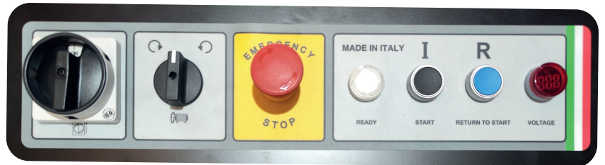
Low voltage of the control electrical panel (24v)
